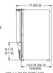
ADD 1-1/2" TO DEPTH FOR WATER LINE CONNECTION
